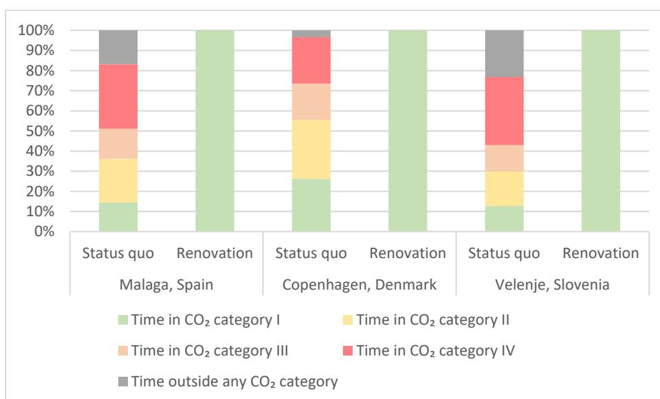
Figure 3. Percentage occupied time in CO<sub>2</sub> categories defined in DS/EN 16798-1 2019.
