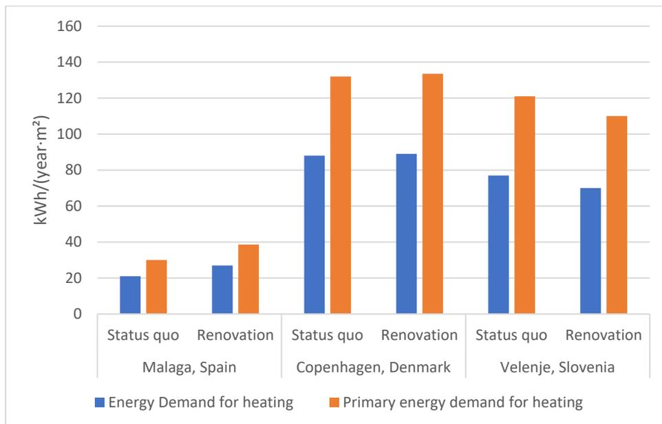
Figure 10. Total and primary energy demand from the energy supply side module.
