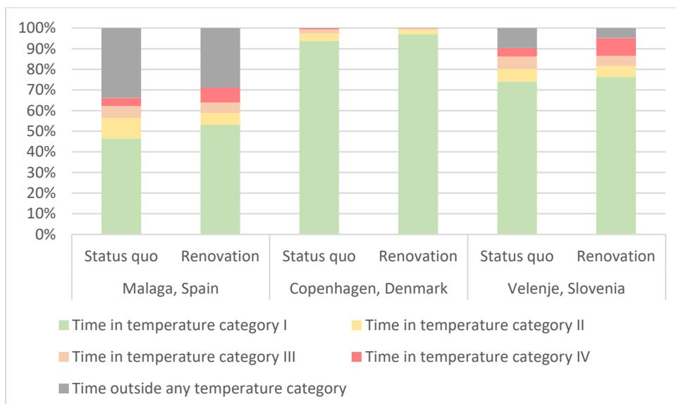
Figure 4. Percentage occupied time in temperature categories defined in DS/EN 16798-1 2019.
